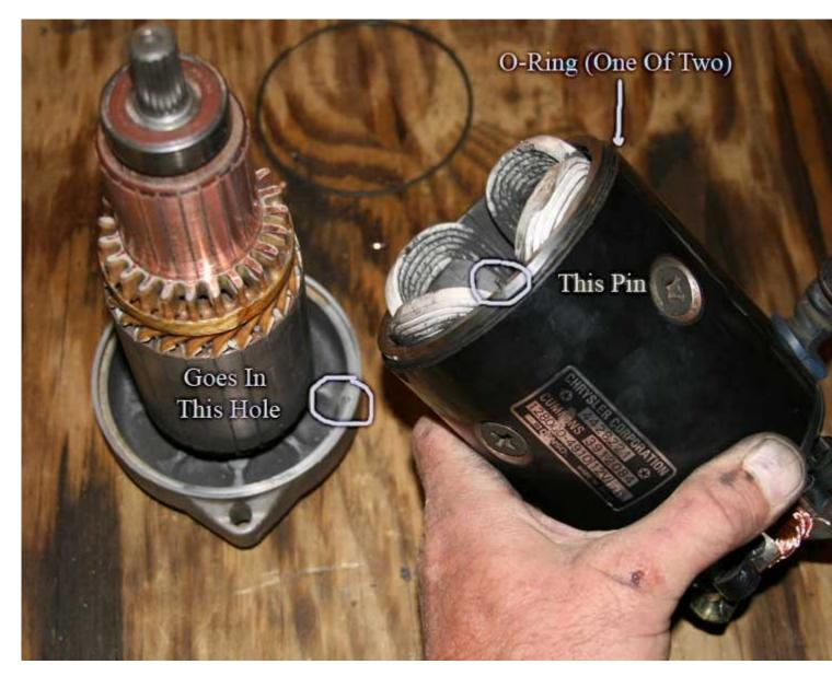
Carefully holding everything, lower the motor housing and brush assembly down over the armature being careful of the brushes as the gear end of the armature come through. Just let it rest there.
