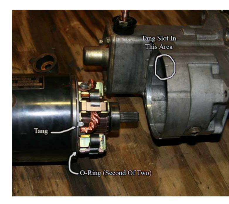
Seeing that things are squarely seated, reinstall the two long bolts and snug them up. Reconnect the motors power cable to its solenoid bolt with the remaining washer and thin nut you had from the solenoid rebuild. Replace the cables rubber boot nice'n purdy.
